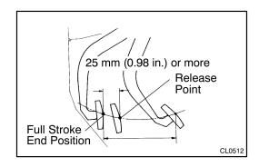
(d) Gradually depress the clutch pedal and measure the stroke distance from the point the gear noise stops (release point) up to the full stroke end position.
