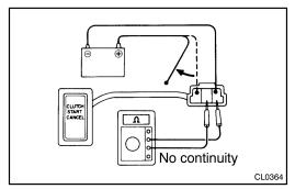
(d) Check that there is no continuity between terminals 1 and 2 when disconnect the battery lead.
