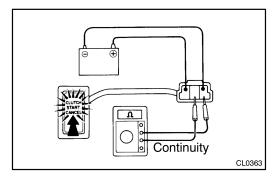
(c) When pushing the switch, check that the indicator light connect on and there is continuity between terminal 1 and 2.
